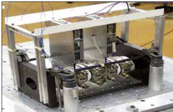
Figure 4. Representative Illustration of an IGCT-based SSCB Mechanical Assembly (Only Power Devices and Heat-sinks, No Snubbers)
