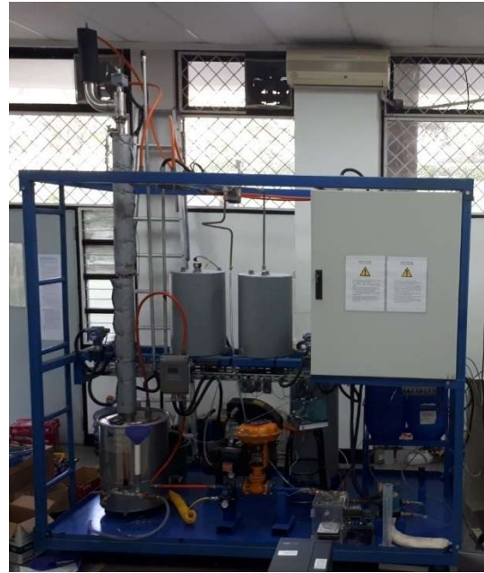
Figure 1. Batch Distillation Column in Honeywell Laboratory of STEI - ITB
