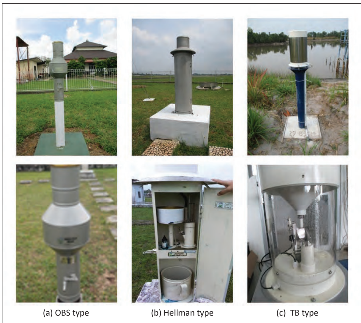
Figure 1. Three Kinds of Rainfall Sensors Installed at field
