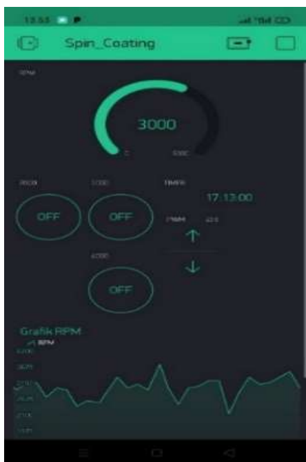
Figure 4. Turning on the spin coating in the Android smartphone application
