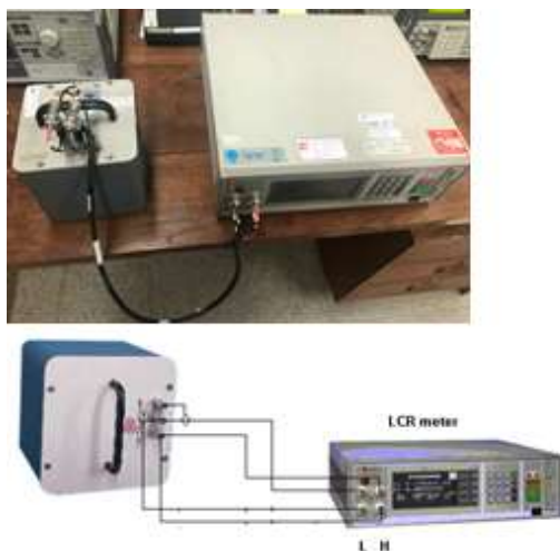
Figure 2. The connection for Inductance Measurement using LCR meter
