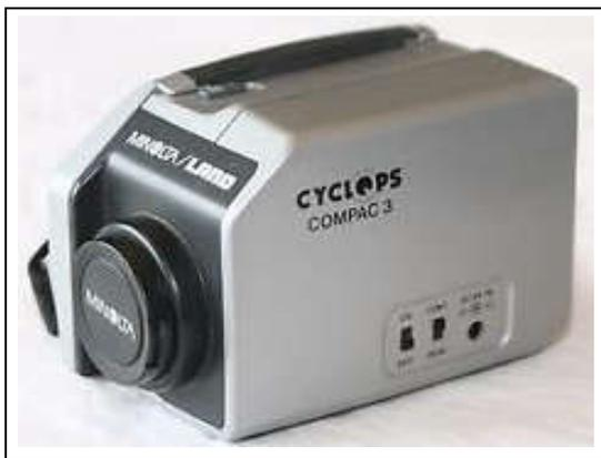
**Gambar 6.** Termometer radiasi standar
